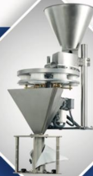
VİDALI DOLUM AUGER FILLING
